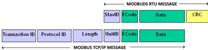
The Modbus commands and user data are themselves encapsulated into the data container of a TCP/IP telegram without being modified in any way. However, the Modbus error checking field (checksum) is not used, as the standard Ethernet TCP/IP link layer checksum methods are instead used to guarantee data integrity. Further, the Modbus frame address field is supplanted by the unit identifier in Modbus TCP/IP, and becomes part of the Modbus Application Protocol header (more on this later).
